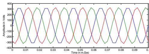
Fig.26. Input waveform for ' $q=0.5$  and Amplitude =325.26 V in 'r' Phase
