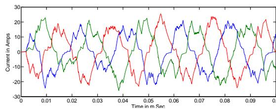
Fig.36. Output Current waveform for 3 phase to 3 phase Matrix converter ('r', 'y', 'b' Phases)
