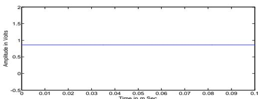
Fig.19. Simulation waveform for Voltage Transfer ratio 'q'=0.866.
