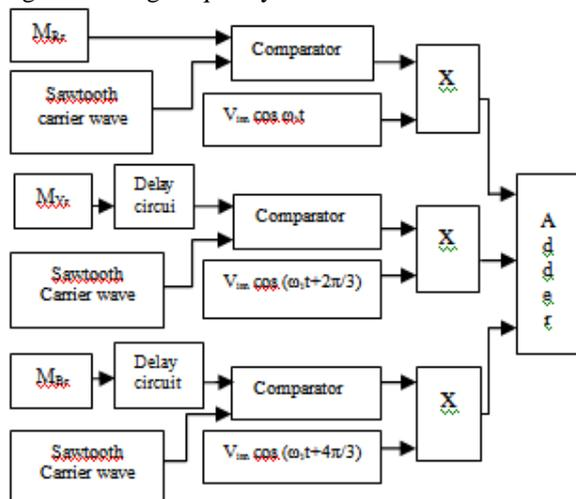
Fig.4. Designing block of power circuit of 'r' phase in 3 phase to 3 phase Matrix converter.
