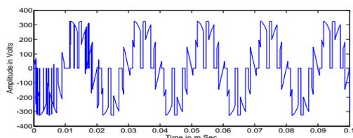
Fig.17. Output Voltage waveform for 'q'=0.866 in 'b' Phase.
