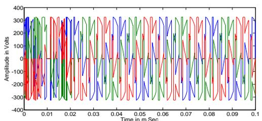
Fig.21. Output Voltage waveform for 3 phase to 3 phase Matrix converter ('r', 'y', 'b' Phases)
