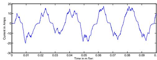
Fig.28. Output current waveform for ' $q=0.5$  in 'r' Phase
