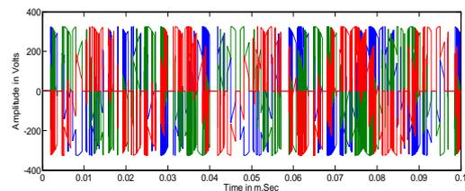
Fig.35. Output Voltage waveform for 3 phase to 3 phase Matrix converter ('r', 'y', 'b' Phases)
