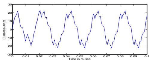
Fig.14. Output current waveform for 'q'=0.866 in 'r' Phase.
