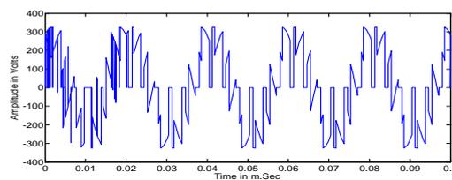
Fig.13. Output Voltage waveform for 'q'=0.866 in 'r' Phase.
