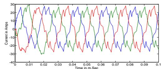
Fig.22. Output Current waveform for 3 phase to 3 phase Matrix converter ('r', 'y', 'b' Phases)
