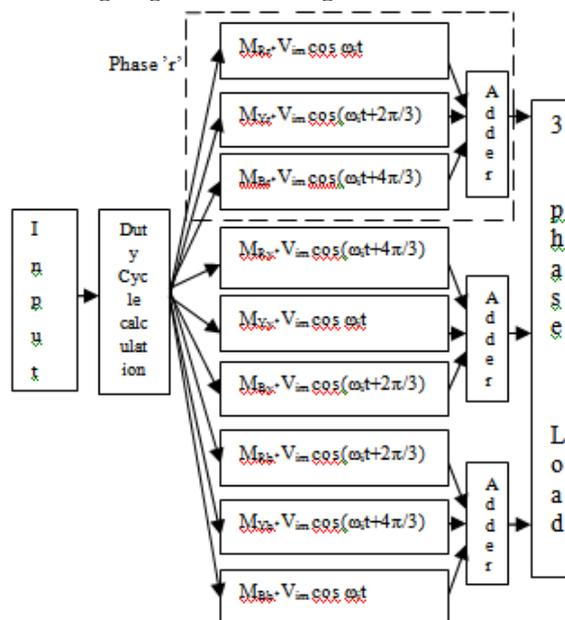
Fig.3. Mathematical Designing of 3 phase to 3 phase Matrix converter.
