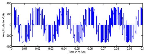
Fig.27. Output Voltage waveform for ' $q=0.5$  in 'r' Phase.
