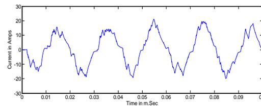
Fig.32. Output current waveform for ' $q=0.5$  in 'b' Phase.
