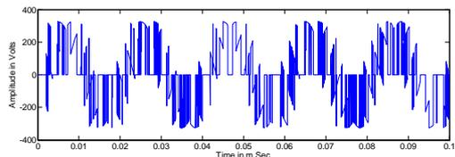
Fig.29. Output Voltage waveform for ' $q=0.5$  in 'y' Phase.
