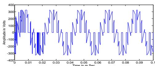
Fig.15. Output Voltage waveform for 'q'=0.866 in 'y' Phase.
