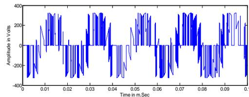
Fig.31. Output Voltage waveform for ' $q=0.5$  in 'b' Phase
